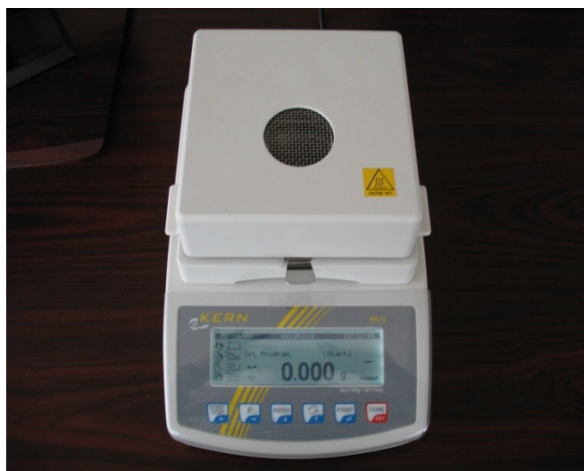
Fig. 1 The Kern MLs thermobalance used for the determination of dry matter
